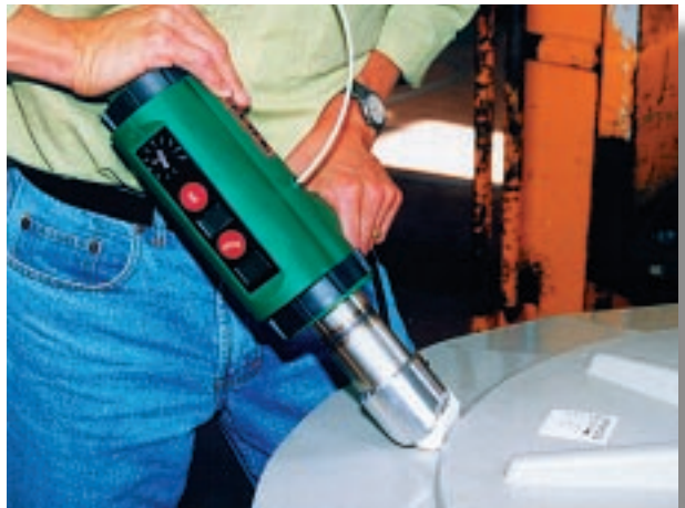
Weldmax Mini-Handextruder being used to weld PP
